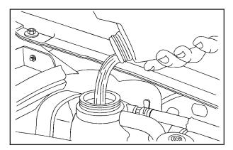
Fill the coolant surge tank with the proper mixture, to slightly above the FULL COLD/FROID line on the side of the coolant surge tank. 4. With the coolant surge tank pressure cap off, start the engine and let it run until you can feel the upper radiator hose getting hot. The upper radiator hose is the largest of the hoses which comes out of the radiator, on the passenger's side of the vehicle. Watch out for the engine cooling fans.
